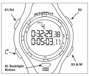
When a Distance or Sample Count Is set In Turbo Set Up mode, "SPD" (Speed) indicator will be illuninated at bottom of display. The number you enter should correspond to the Distance or Sample Count you want to use for the Speed or Rate Computation. "P-HR" in display means watch is set to compute "per Hour" rate, and "P-Mn" means watch is set to compute a "per Minute" rate.
